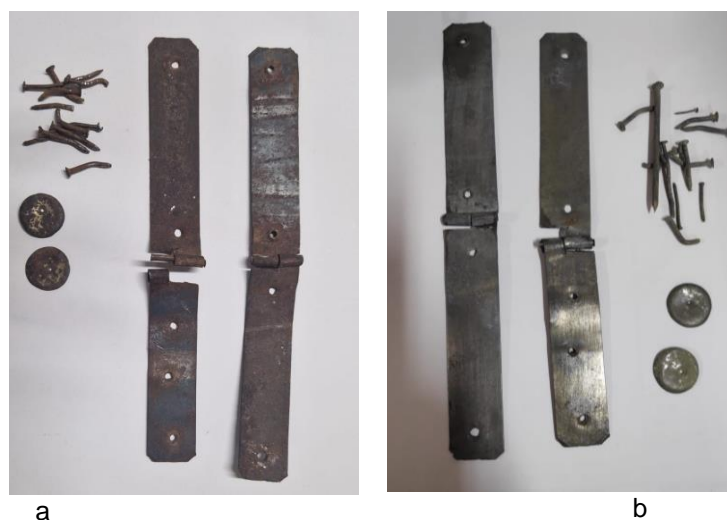
Fig. 13. Metal elements before (a) and after cleaning (b).
